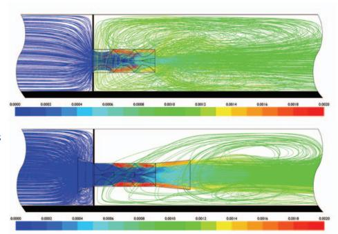
Pathlines Colored by Volume Fraction of Injected 4000 Mixer (above) and the Inlet & Diffuser (below)
